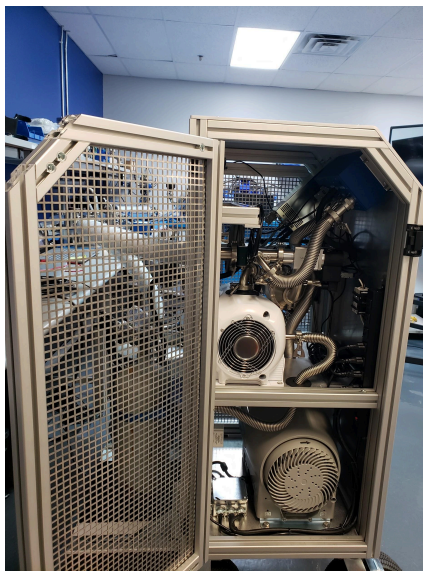
Figure 2. - Photo of inside of the Cart, featuring rough/backing pumps and various hardware.
