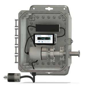
**Reminder**: The internal volume of this gauge has been evacuated and backfilled with nitrogen several times to avoid moisture or humidity concerns. If the enclosure is opened up, this process needs to be repeated again to mitigate any moisture concerns.
