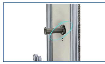
Connect the cart to your system via KF40 connection. \*Note: Smooth connections are better for flow.
