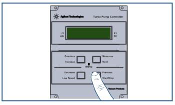
Press "Start" on the Turbo Controller and wait 5 minutes for it to spin up.
