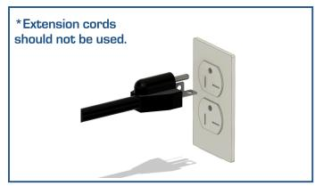
Plug cart into a 20 amp 110V receptacle outlet. \*Note: Only the cart can be plugged into the outlet, no other devices.
