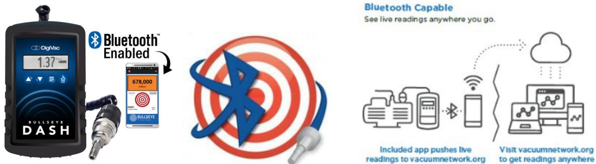
The Bullseye DASH can be ordered with a Bluetooth module, which interfaces with the [Vacuum Gauge Application](#) for remote, real-time vacuum monitoring and graphing through a phone or tablet. The vacuum data can then be read and exported via [vacuumnetwork.org](#) to a .csv file and shared. The app can be found by searching “[Vacuum Gauge](#)” in the [Apple Store](#) or [Google Play Store](#). The app range is up to 300 feet under ideal conditions.
