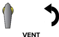
The chamber pressure gauge will count upward to 0 inHg.
