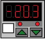
As set at the factory, this gauge shows the chamber vacuum level in inches of mercury (inHg) relative to sea level atmospheric pressure. The display range is 0 to -29.9 inHg. Zero is the room atmosphere pressure at sea level and -29.9 inHg a near-perfect vacuum. See page 44 for how to display other units of measurement or zero the gauge to your local altitude.
