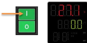
Place the oven **Power Switch** in the ON ( I ) position.
