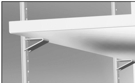
1. Install the shelf clips in the slots of the shelf standard mounting rails located on the sides of the chamber interior, 4 clips per shelf.
