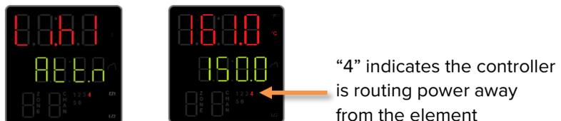
Alternating alert screens flash when the high limit heating cutoff is active.
