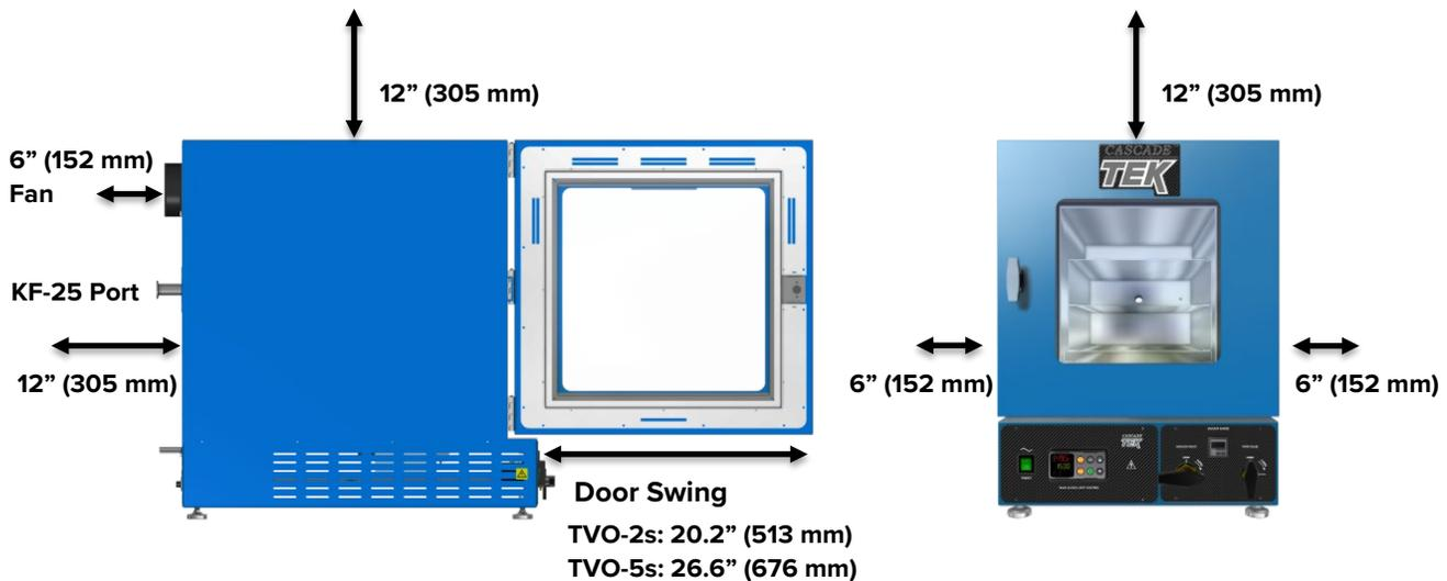
**6 inches (152 mm)** of clearance is required on the sides.
