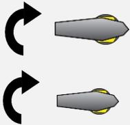
Verify the oven **chamber door** is **closed and latched**, and that the **vent intake valve** and **vacuum valve** are in the **closed position** (turned all the way clockwise).
