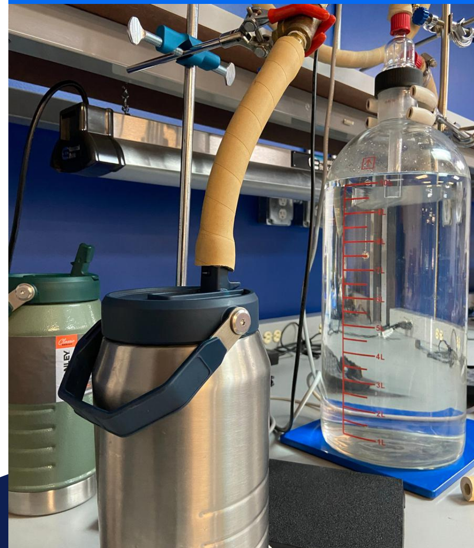
Vacuum Leak Detection by Simulating Human Suction
