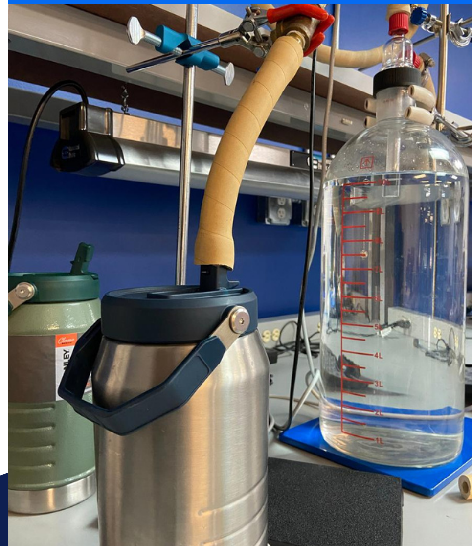
Vacuum Leak Detection by Simulating Human Suction
