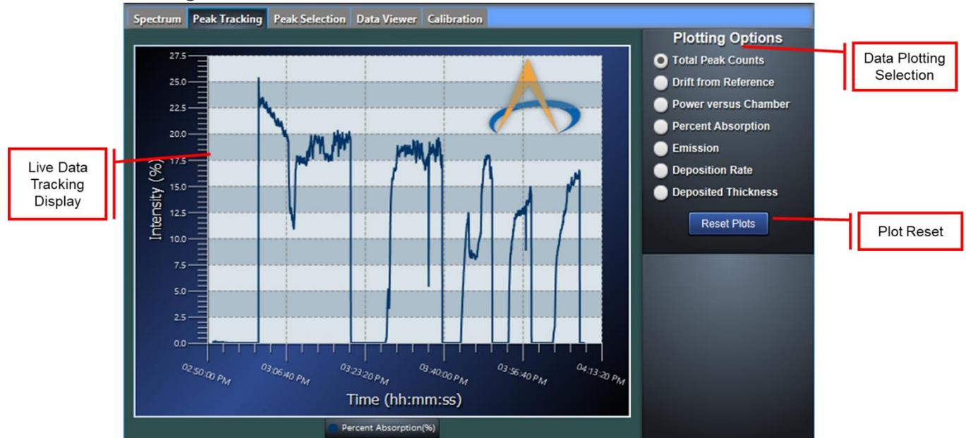
The peak tracking tab is the main tab for monitoring a process with the AtOMS system. The software provides a variety of ways to view the data. The panel includes data tracking options which can be selected with the radio button on the right. The plotted data can be reset by using the “Plot Reset” button on the right side of the panel.
