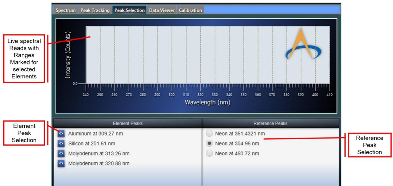
The Peak Selection Tab allows the user to select which elements to monitor as well as which reference peak to use. To change which elements are being monitored, toggle the “eyeball” next to each elemental line.
