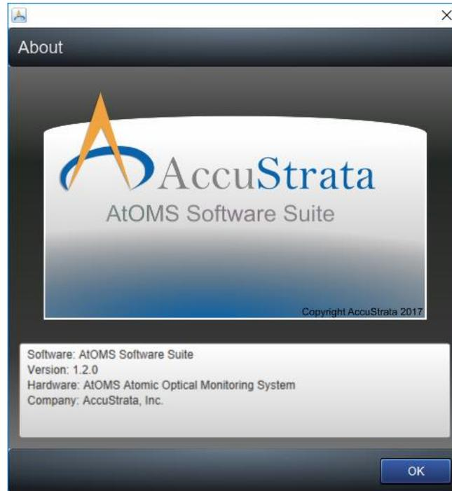
The About menu is used to identify critical versioning information about the software. To ensure that updates have been correctly implemented, use the Version number.
