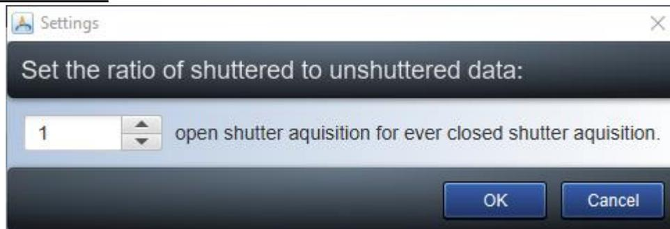
**Shutter Ratio** is the number of times a reference read will be reused. A setting of 1 will take a new reference reading for every measurement. This is the recommended setting and should only be changed
