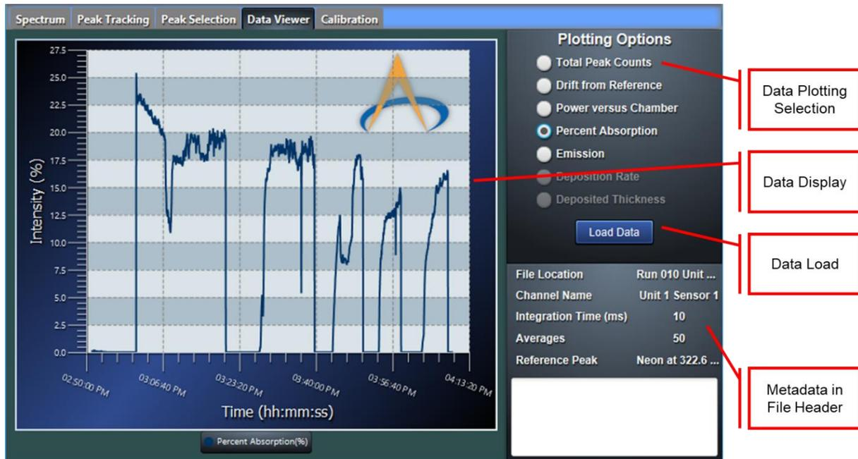
The Data Viewer Tab allows users to review old runs. The user can select between each of the plots by using the “Plotting Options” radio buttons. The metadata about the run including filename, sensor information, integration time, number of averages and the reference peak used for the data as well as any comments saved by the user will be displayed in the “Metadata” section. To load data, press the “Load Data” button and select the desired file.
