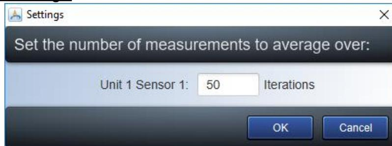
The **Scans to Average** is used to increase statistics for the measurement and improve the signal to noise; however, increasing the number of scans will also increase the data acquisition time. Users should balance the number of scans with the rate at which the processes are being monitored (sampling rate).
