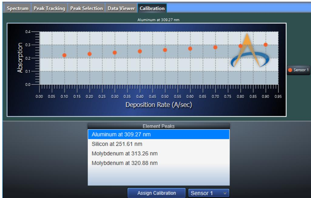
The Calibration tab is used to provide calibration curves that can be used to convert atomic absorption to deposition rate and thickness. To assign a calibration file to a specific elemental peak:
