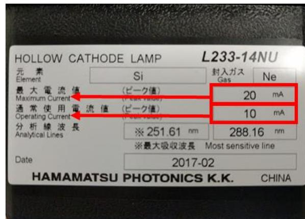
*Warning: Incorrect power settings for a lamp can lead to decreased lamp lifetime or catastrophic lamp failure. Use caution when setting up the lamp.*
