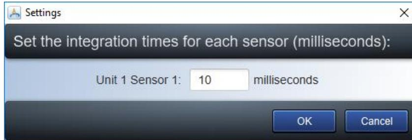
The **Integration Time** is the amount of time over which the detector will collect light. The higher the integration time, the higher the total peak counts will be. The detector generally is most sensitive with counts around 40,000; however, other factors such as reference peak intensity and lamp power may affect this.
