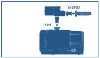
Mount the DINAMO valve between the vacuum pump and the system.
