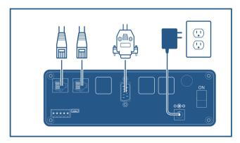
Connect the sensor cable(s), valve cable, and power supply to the rear of the FRYA controller.
