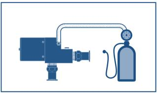
(Optional) Connect nitrogen or other inert gas to the DINAMO valve's hose barb. Leave alone if venting with ambient air.
