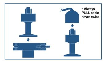
Mount the sensor(s) into the vacuum system and attach sensor cable(s). Make sure to use properly labeled cable and port.
