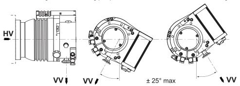
Fig. 5: Recommended alignment when using oil-sealed backing pumps
