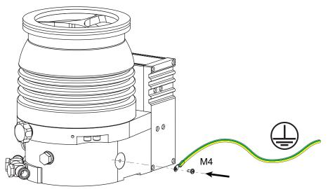
Fig. 17: Example: Connecting the grounding cable
