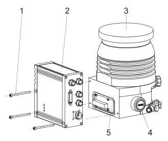
Fig. 22: Installation of electronic drive unit TC 400
