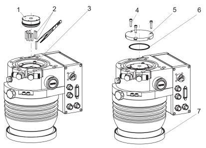
Fig. 20: Installing the operating fluid reservoir
