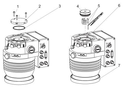
Fig. 19: Removing the operating fluid reservoir
