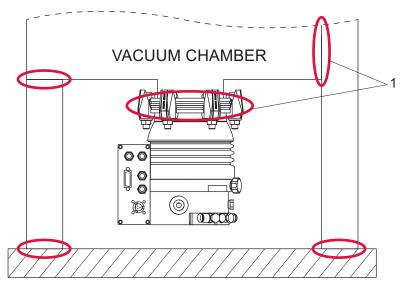
Fig. 4: Example: Safety connections
