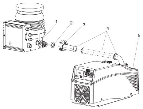
Fig. 16: Example of fore-vacuum connection on HiPace 300
