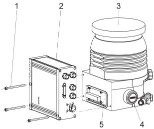
Fig. 21: Removal of electronic drive unit TC 400
