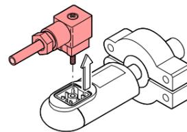
**4** Remove the gauge from the vacuum system.
