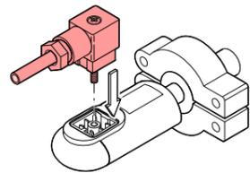
**3** Connect the sensor cable to the controller.
