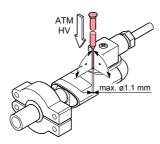
Evacuate to p  $\ll 10^{-4}$  mbar (recommended) or to a pressure in the range of 10<sup>-4</sup> ... 10<sup>-2</sup> mbar and wait at least 2 minutes.
