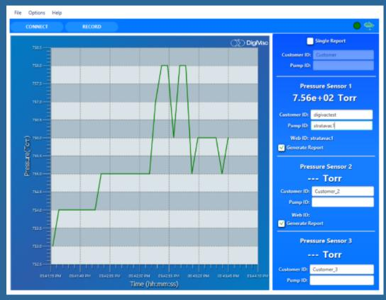
Assign each sensor a dedicated customer ID and a unique pump ID. You can also select whether you need individual sensor reports (each .csv file and pumpdown curve illustration shows the readings of the selected sensor only) or a single report (where the .csv file and pumpdown curve illustration show the behavior of all sensors connected to the gauge).
