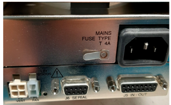
TwisTorr Medium-TMP onboard controller for TwisTorr 404 FS, 704 FS, and 804 FS turbo pumps
