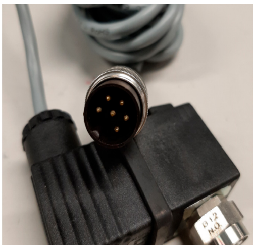
Vent Valve Circular connector 1.2 mm ID – N.O/N.C
