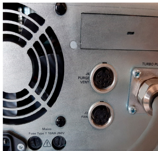
TwisTorr Medium-TMP rack controller for TwisTorr 404 FS, 704 FS, and 804 FS turbo pumps.
