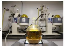
The cannabis market uses three main extraction techniques: CO2, liquefied hydrocarbons, and ethanol extraction. In all processes, the plant material is subjected to a solvent to remove active compounds from the plant matter and filtered to yield a solution of the solvent with plant extracts.
