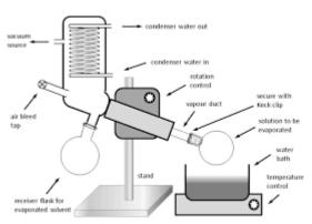
Typically, the distilling flask is filled to 50% volume. The water bath is heated to  $30-40^{\circ}$ C. The condenser temperature, controlled by a recirculating chiller, is set to  $-10^{\circ}$ C to  $0^{\circ}$ C. Once the water bath and condenser have reached the set points, the distillation flask is rotated from 150-200 rpm.
