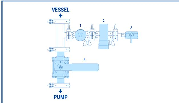
Configure the (1)DCP, (2)CONVECTRON, (3)VENT VALVE, and (4)ISOLATION VALVE between the VESSEL and PUMP as pictured
