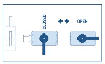
Flush the sensors by opening the VENT VALVE briefly and close
