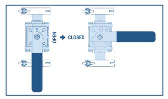
Isolate the vessel by closing the ISOLATION VALVE
