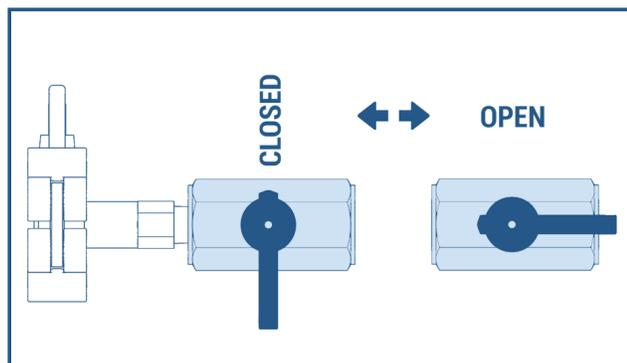
Flush the sensors by opening the VENT VALVE briefly and close
