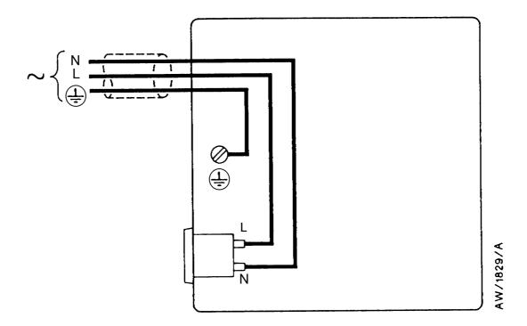
Figure 3 - Electrical supply connection, single-phase motors:  $220\text{-}240\ V\ 50\ Hz\ and\ 230\text{-}240\ V\ 60\ Hz$
