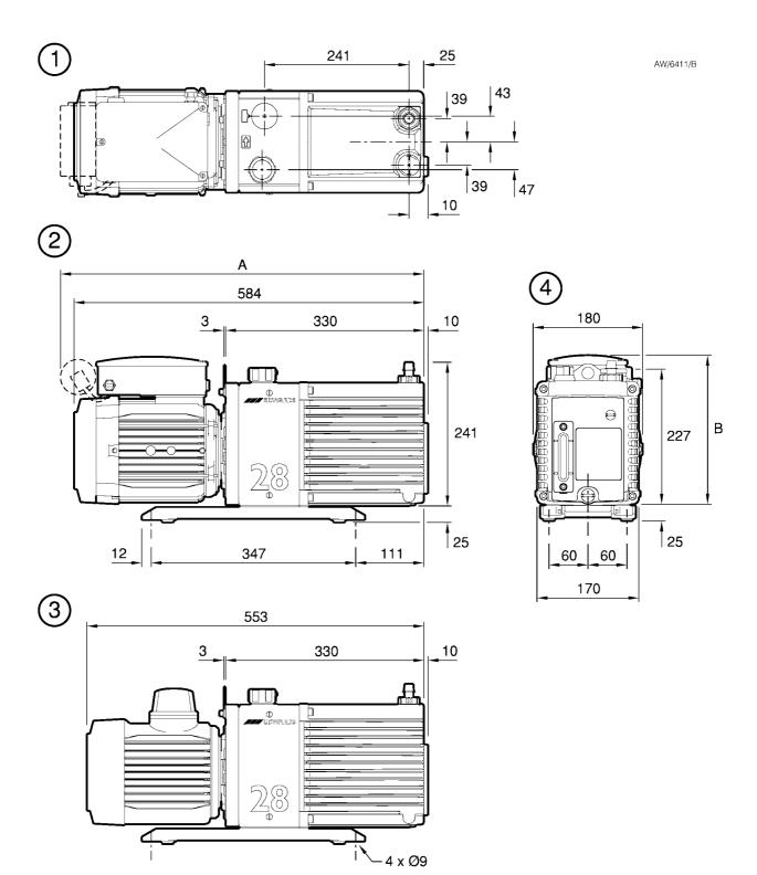
Figure 2 - Dimensions (mm)
