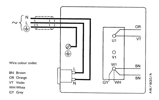
Figure 4 - Electrical supply connection, single-phase motors:  $100\ V\ 50\ Hz,\ 100\text{--}105\ V\ 60\ Hz\ and\ 115\ V\ 60\ Hz$
