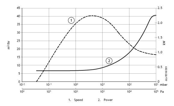
**Note:** The pump is not suitable for prolonged operation at inlet pressures above 40 mbar. Under such conditions, the inverter may reduce the motor speed.
