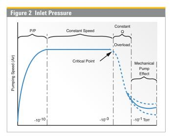
Typical plot of diffusion pump performance. Four regions are evident: 1) Effect of the pressure ratio limit; 2) Normal operating range with constant speed; 3) Throughput limited condition; 4) Effect of backing pump.
