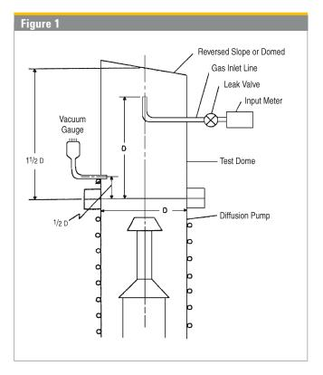
period is considered. All backstreaming tests were perfomed using DC-704 pumping fluid (no longer available).
