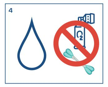
When clean of contaminants, the solvent should run clear out of the sensor tube. Let the sensor air dry. Do NOT dry the sensor after cleaning with compressed air or a cotton swab.
