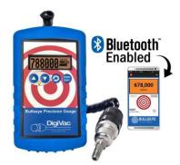
**Vacuum Measurement and Monitoring**: The **Bullseye Precision Gauge with Bluetooth** has patented vacuum graphing and has become the standard for measuring SPD processing. Combine with the **Vacuum Gauge App** to enable remote monitoring. Set low and high alarms plus email data, and graphs for process improvement.
