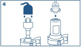
Connect sensor cables to sensors. Make sure to use properly labeled cable and port.
