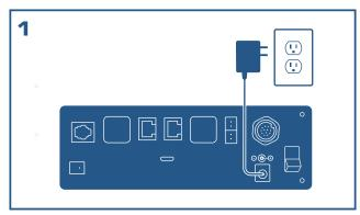
Connect the display, connect the power supply to the unit and wall. Verify that StrataVac powers on then power off.
