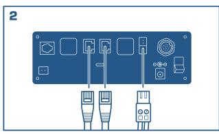
Connect the sensor cables and valve relay cables to StrataVac ports.
