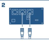
Connect the sensor cables to the StrataVac.
