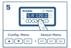
To assign the sensor type to the corresponding slot, enter the configuration menu (UP, DOWN, ENT). Then navigate to the sensor selection menu (ENT, ENT, SEL).
