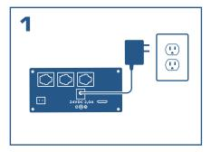
Connect power supply to unit, then connect to power supply to wall. Verify that StrataVac powers on.
