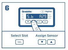
From sensor selection menu, use "SEL" to switch between slots. Then use the arrows to navigate to the appropriate sensor type for the slot
