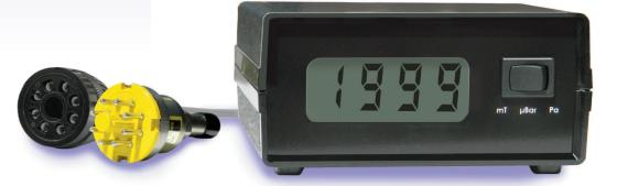
**The Model 100H** is a portable digital vacuum instrument that reads from 1 milliTorr (1 x 10^-3 Torr) up to 1999 millitorr/microns and comes standard with a Hastings DV-6M thermocouple vacuum gauge tube.
