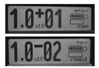
The numeric display shows the currently configured units, in these examples the vacuum pressure units are "microns" or "torr".
