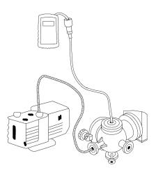
pinpoint leaks If you have a leak, start with the pump. If the pump works, start adding components until you find the leaky one, then fix. Retest. Here is an example of leak testing.
