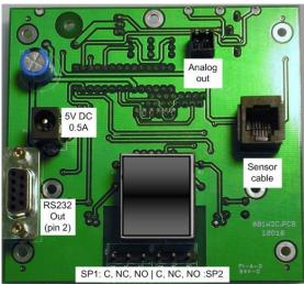
The set point connections are in the back of the unit. There is one row of pins with a terminal strip connector for the 2 set point connections. The set point connections are in the order:
