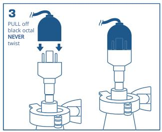
Connect the octal end of the sensor cable to the vacuum sensor
