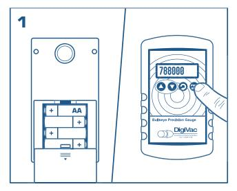
Install batteries or Connect to USB, press power button and verify that the display lights up
