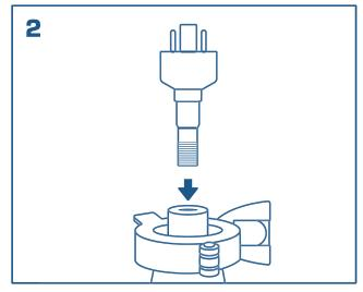
Plumb the thermocouple gauge in your vacuum system, making sure to orient the sensor vertically so the threads are down. This is for best accuracy and long term reliability.
