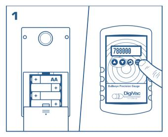
Install batteries, press power button and verify that the display lights up
