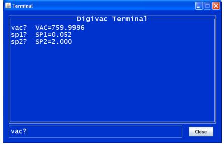
Press return or enter to submit the query or change the set point. Note that while the web terminal is open, the main 2L760 screen will not update. If at any time the web terminal or the main 2L760 applet window becomes unresponsive, close the.
